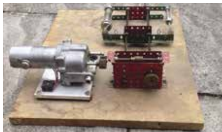
Infusion pump made from Meccano used in physiology experiments in the 1960s
